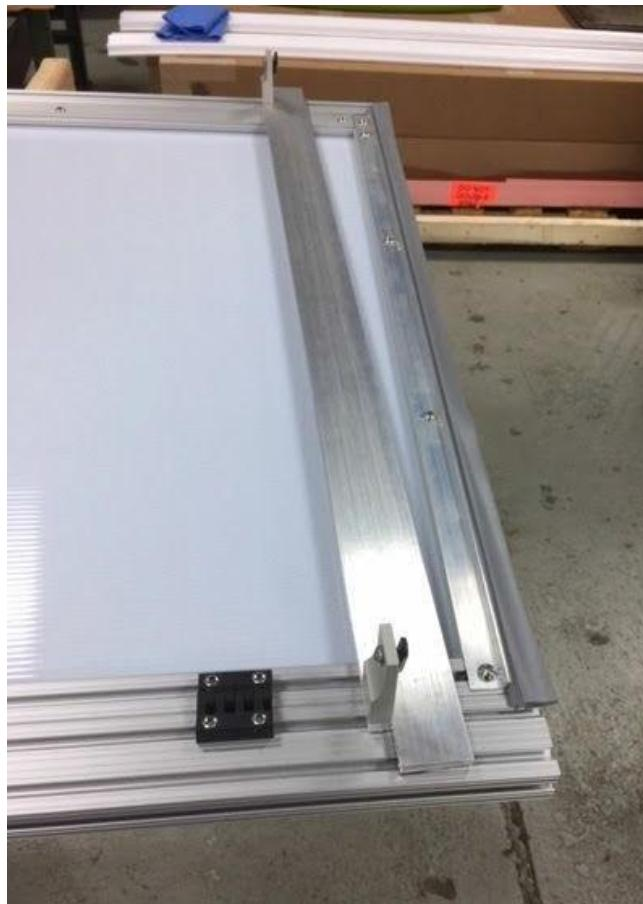
✖ **STEP THREE:** Remove the door sweep. Remove the 6 button-head screws that hold the sweep in place. Remember to save the 6 screws and the 2 black oval-nuts that will slide out of the 2 channels, you will need them for Step 7. Note the remaining 4 black oval-nuts will remain in the channel for future use if you wish to return the door to its original height.
