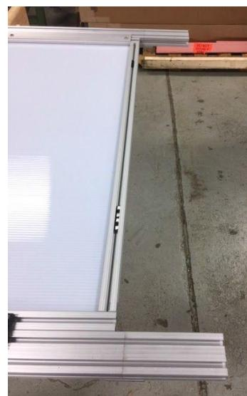
**✖ STEP FIVE:** Add the extension panel to the bottom of the door with 4 mini clamps. Line up the extension panel with the door. The black, oval nuts should be in the lower channel, facing up (you will need these to reattach the door sweep in Step 7). Begin with 2 mini clamps on the front side but do not tighten them too much. On the underside, place a mini clamp directly behind each mini clamp on the front side. Alternately tighten the clamps until the panel is secure and even.
